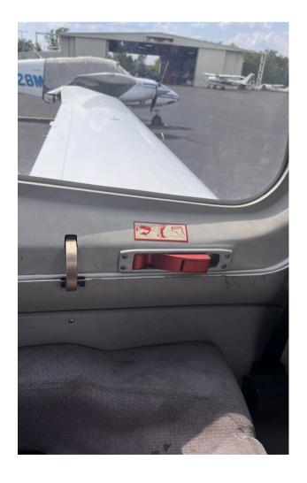
Shortly after takeoff a DA-40 Crew noticed a Door Warning annunciation. The crew visually inspected the back door and realized that the rear door "was hanging on to the lip caught by the safety catch that is on the inside of the door." The crew immediately returned to land and made a soft field landing. On touchdown, the door came open completely and detached from the aircraft.
